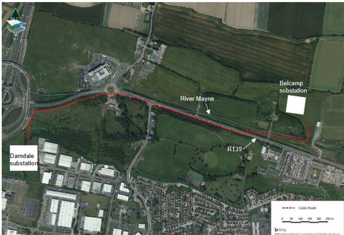
Figure 1 Proposed Route of the underground cable installation
